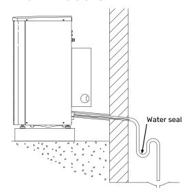
The condensation water is lead to an indoor drain (subject to local rules and regulations).
