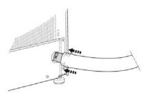
7. Secure the insulation with a cable tie.
