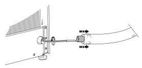
5. Lay the heating cable and ensure that the marking on the heating cable is as close to the condensation water connection as possible. Secure the heating cable with cable ties to the top of the evaporator, as illustrated in point 9.
