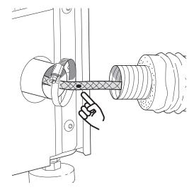
6. Connect the hose to the condensation water connection and tighten the hose clamp. Pull the insulation up towards the plate.
