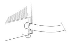
8. Route the heating cable to the electrical connection.
