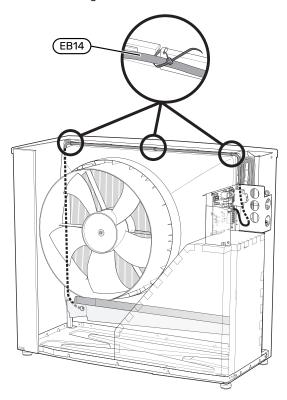
10. Connect the cable as illustrated in "Electrical connection", see page Electrical connection. (Check the fuse according to the table, see page "Fuse".)
